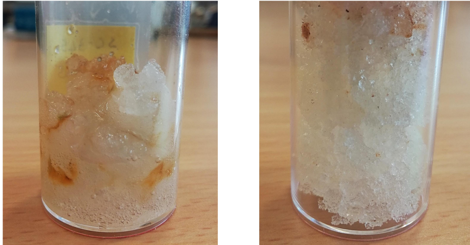
Fig. 10. Appearance of the PEG-free sample ( \text{CaCl}_2/\text{SiO}_2 ) after sorption #5: material retrieved from the (left) lower part and (right) upper part of the reactor
