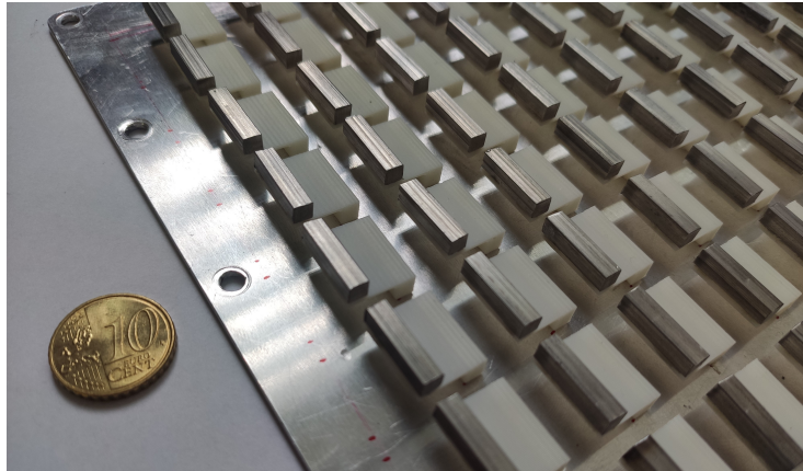
Figure 18: Close-up view of the LRM Plate (aluminium plate with 72 ABS-Steel micro-resonators) next to a 10 cent euro coin (for scale perception).
