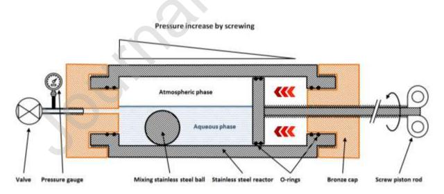
Figure 4: Schematic view of a screw-piston reactor (adapted from Schedler, 2016).
