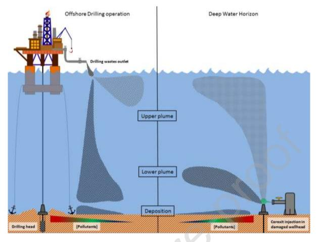
**Figure 2:** Schematic representation of the similarities between idealized plumes and deposition between deepwater offshore drilling operation and DWH hydrocarbon propagation post blowout.
