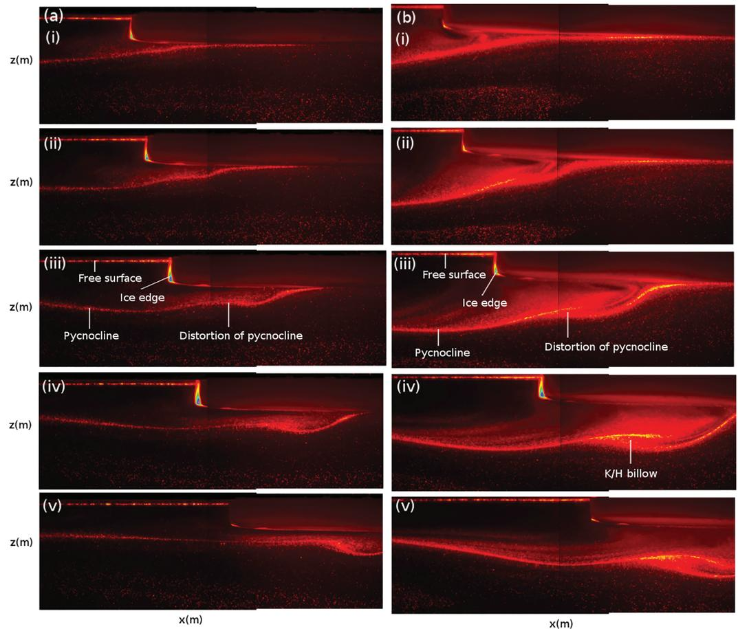
**Figure 4.** Series of experimental images for an experiment in which the ice was level ice of dimensions  $d_f = 0.058$  m and  $l_f = 1.00$  m, and the incident ISW had (a)  $a = 0.053$  m and (b)  $a = 0.113$  m. The images show light intensity and ordered sequentially in time from top to bottom at intervals of  $\Delta t = 2.14$  s; subpanel dimensions are  $(\Delta x, \Delta z) \approx (0.813$  and  $0.74$  m). The ISW propagates from left to right.
