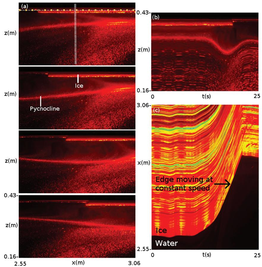
**Figure 2.** (a) Series of still experimental images with level ice of dimensions  $d_f = 0.013$  m and  $l_f = 0.95$  m, showing light intensity, ordered sequentially in time from top to bottom at intervals of  $\Delta t = 2.2$  s, (b) vertical time series made from column marked by vertical dashed line in (a), and (c) horizontal time series made from row marked by horizontal dot-dashed line in (a) rotated through  $90^\circ$  anticlockwise.
