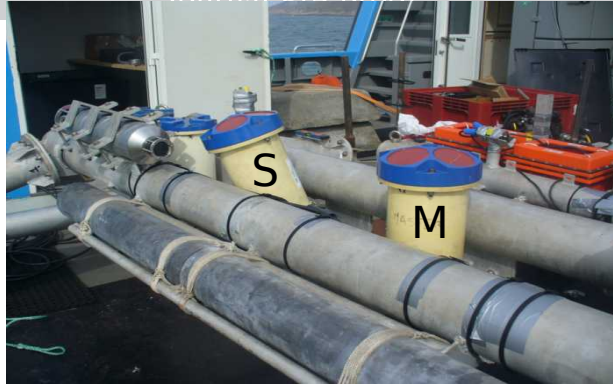
Figure 2: Master (M) and Slave (S) ADCP mounted on the frame prior the deployment.
