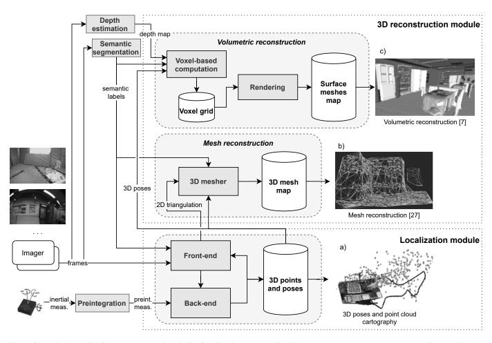
Fig. 1. Conventional real-time 3D scene reconstruction pipeline from imaging sensors and inertial measurements. a) represents an accurate trajectory estimation and a sparse point cloud scene representation. b) corresponds to the visualization of a 3D mesh introduced in [27]. c) is the volumetric voxel-based reconstruction provided by [7].
