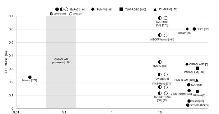
Fig. 2. Comparison of state-of-the-art methods in terms of accuracy and range of power consumption (W) between several hardware platforms, from ASIC to CPU-based. The vertical axis corresponds to the average RMSE in meters in all successful dataset sequences provided by the authors. Methods denoted by (\*) means that the error has been obtained from [5].
