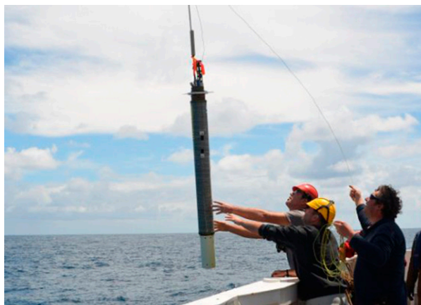
FIG. 11. Deep-Arvor deployment during Geovide cruise, May 2014. The float is suspended by its damping collar with a handling rope and then launched at the sea surface by means of a trigger snap shackle.
