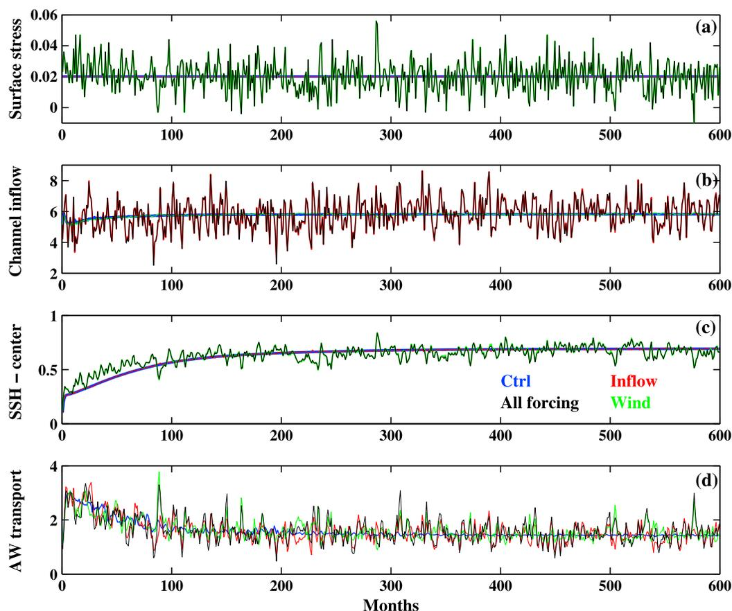
**Figure 4.** Time series for the four sensitivity experiments performed with the idealized model of (a) the surface stress (in  $\text{N m}^{-2}$ ), (b) the inflow through the channel (in Sv), (c) the SSH at the center of the circular basin, and (d) the transport of the AW current (in Sv).
