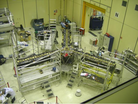
Fig. 1: SMOS in the EADS-CASA Espacio test facilities. The three-arm antenna, folded for launch, measures 8 m in diameter. The choice of L-Band requires novel technology to be flown in space, which has been realised with SMOS for the first time. With the antenna size being proportional to the wavelength, synthetic aperture and interferometric processing were required for a space application.
