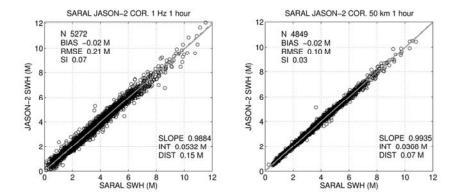
Figure 8 : SARAL Jason-2 SWH comparison: 1 Hz (left) and 50 km along-track average (right) collocated data within 1 hour time window.
