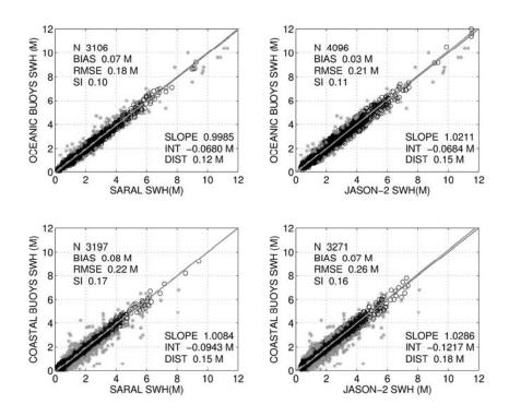
Figure 6: SARAL (left) and Jason-2 (right) SWH comparison with buoy data, for open ocean buoys (top) and coastal buoys (bottom).
