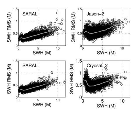
Figure 11: comparison of 1 Hz SWH rms as a function of SWH, for collocated data set: SARAL Jason-2 (top), SARAL Cryosat-2 (bottom). Mean value of rms per SWH 0.1 m bins, in grey. 118x88mm ( $300 \times 300$  DPI)
