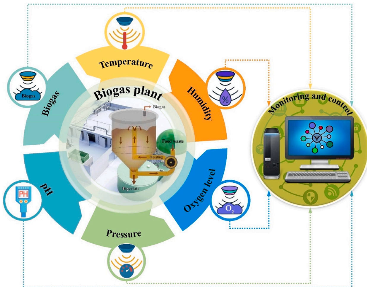
Fig. 4. The Internet of things-based system for managing the food waste valorization process.
