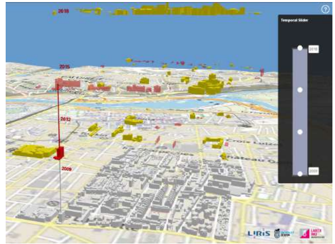
Fig. 7: An example of the STC integration with the use case of Gratte-ciel district (Lyon/France). One building has been selected and the capture show the full temporal transactions linked to that building. The building has remained unchanged from 2009 to 2012 (gray link), an destroyed in 2015 (red link).
