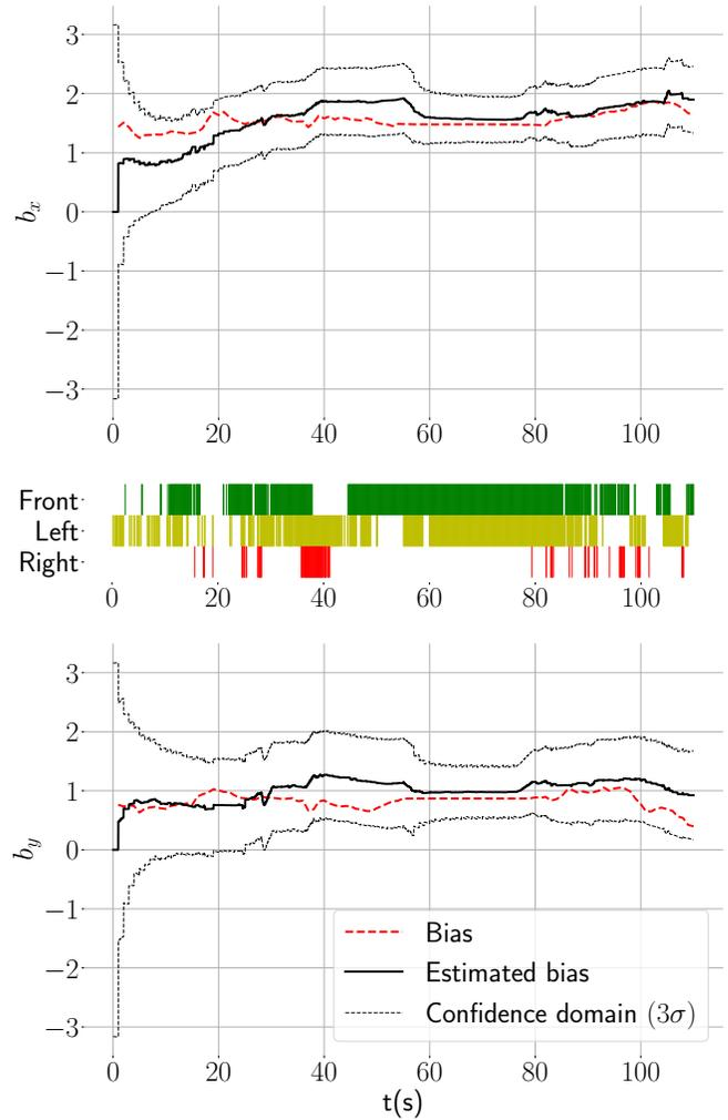
Fig. 8: Biases in ENU frame obtained using the all cameras solution on the 07-06 sequence. Biases on  $x$  and  $y$  axes are respectively on top and bottom. The observations timestamps provided by the different cameras are summarized in the middle (Front camera in green, left camera in yellow and right camera in red).
