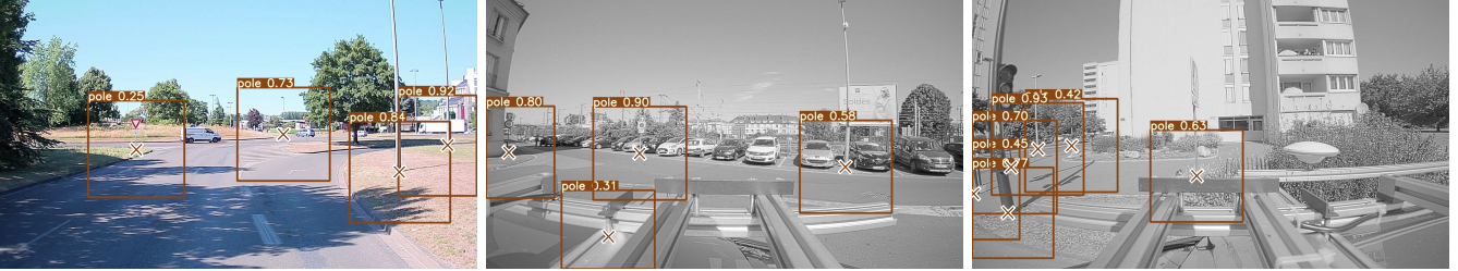
Fig. 3: Examples of detections obtained from YOLOv7-based pole detectors on RGB and grayscale images. Each bounding box is displayed with its detection score and its center corresponding to a pole base is highlighted by a cross. For the grayscale side cameras, a final filtering is applied to remove detections on the vehicle roof.
