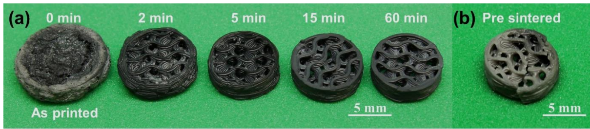
Figure 5: Optical image of the UHSed (a) chemically debinded samples at different soaking times in acetone at 40 °C. (b) pre-sintered sample. UHS experiments was carried out at 26A for 120s.
