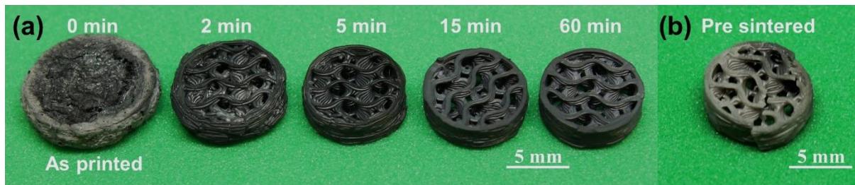
Figure 5: Optical image of the UHSed (a) chemically debinded samples at different soaking times in acetone at 40 °C. (b) pre-sintered sample. UHS experiments was carried out at 26A for 120s.
