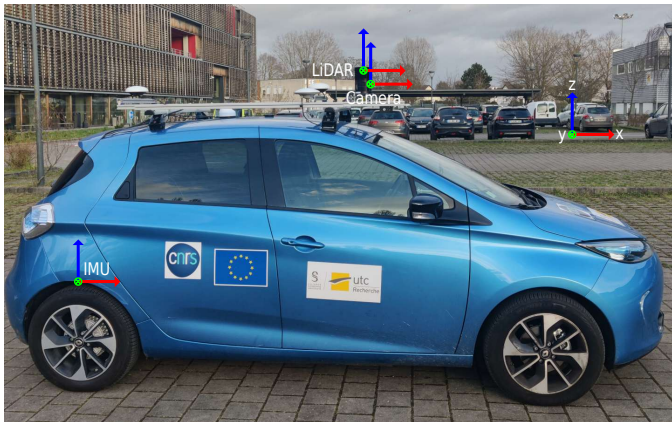
Fig. 6: Experimental Renault ZOE vehicle equipped with a NovAtel SPAN-CPT GNSS/IMU and a Hesai Pandora sensor.
