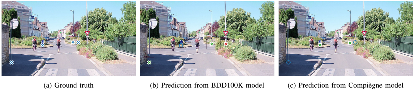
Fig. 8: Ground truth and predictions from models trained on BDD100K and Compiègne on a Compiègne validation image. The green crosses are true positives, red ones false negatives and the blue circles are misdetections.
