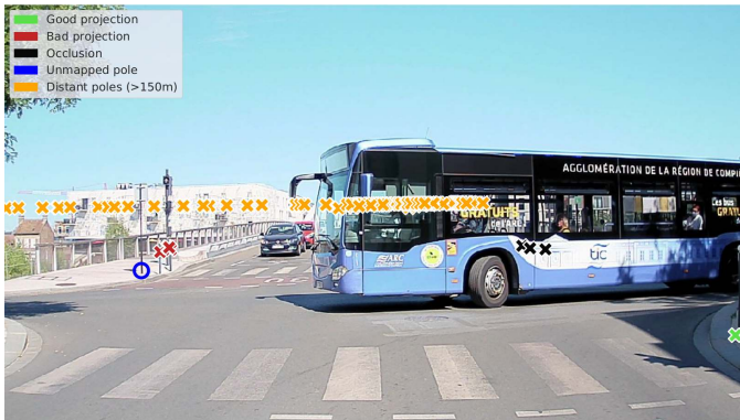
Fig. 2: Naive projection of map features onto an image frame. Only the green point on the right-hand side can be considered as a correct annotation.
