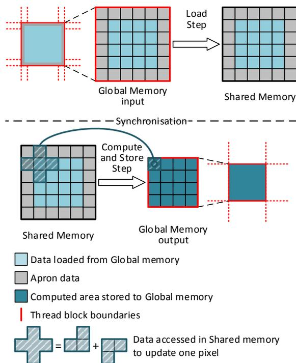
Fig. 5: **Shared\_fusion** thread block memory access pattern for 1 iteration. All the data needed to compute one iteration is loaded in Shared memory. The computation step is then performed using only Shared memory. Finally, the results within the red area are written into Global memory.
