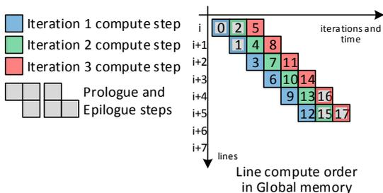
Fig. 6: `Global_pipeline` thread block computer order for the steady-state of a 3-iteration pipeline on 6 consecutive lines. The thread block computes a full iteration on each entire line.
