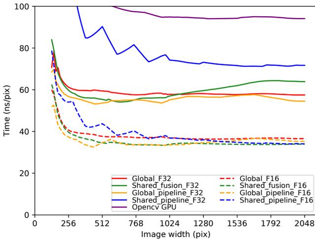
Fig. 10: Execution time (ns/pix) of TV-L<sup>1</sup> implementations on Nano.
