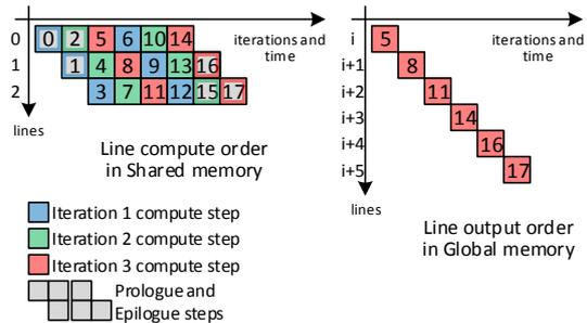
Fig. 7: `Shared_pipeline` thread block compute order for the steady-state of 3 pipelined iterations on 6 consecutive lines. This pattern is run multiple times with an offset for lines wider than the thread block width.
