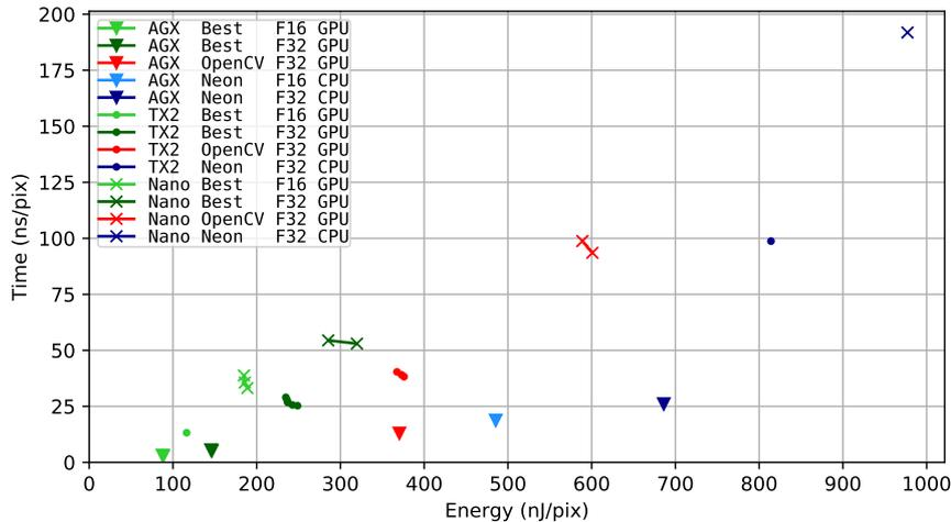
Fig. 12: Time (ns/pix) and energy (nJ/pix) operating points for several TV- $L^1$  implementations on each Jetson boards. Several clock frequencies are tested for each versions for a  $2048 \times 2048$  pixel image.
