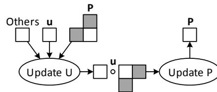
Fig. 2: Inner iterative steps of the TV-L<sup>1</sup> method after operator fusion.
