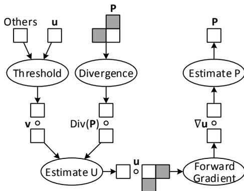
Fig. 1: Iterative steps of the TV-L<sup>1</sup> scheme before operator fusion. This consumer/producer representation highlights the data dependencies of each subsection of the iterative scheme. Operators are centered on the white square and the spatial dependencies shown in gray.  $\circ$  symbolizes function composition i.e. the output of a step is the input of the next.
