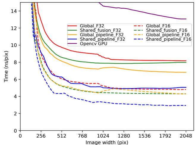
Fig. 8: Execution time (ns/pix) of TV-L<sup>1</sup> implementations on AGX.
