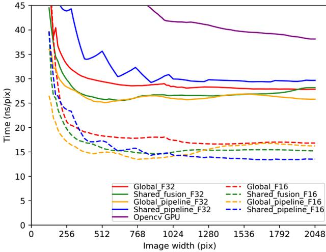
Fig. 9: Execution time (ns/pix) of TV-L<sup>1</sup> implementations on TX2.
