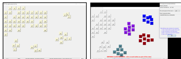
Figure 1: Depiction of the TCL-LabX GUI. (left) Free categorization (1 st step): the sonic icons of the corpus appear as boxes in the interface that the participant has to move in the screen space to form the perceptual categories. (right) free verbalization (2 nd step): each group of sonic icons is selected and labelled and a prototype sound per category is chosen.
