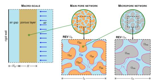
Fig. 1. Generic scheme for acoustic analysis of the double-porosity media. The periodic  $\Omega_{ps}$  domain (the periodic  $\Omega_{ms}$  domain) is marked in orange (grey) and additionally with appropriate labels, and can be compact in 3D. (For interpretation of the references to colour in this figure legend, the reader is referred to the web version of this article.)
