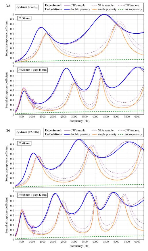
Fig. 10. Predicted and measured sound absorption for single- and double- porosity samples (backed with a rigid wall or an air gap) with a periodic cell size of  $\ell_p = 4 \, \text{mm}$  and a height of: (a)  $H = 36 \, \text{mm}$ , and (b)  $H = 48 \, \text{mm}$ .
