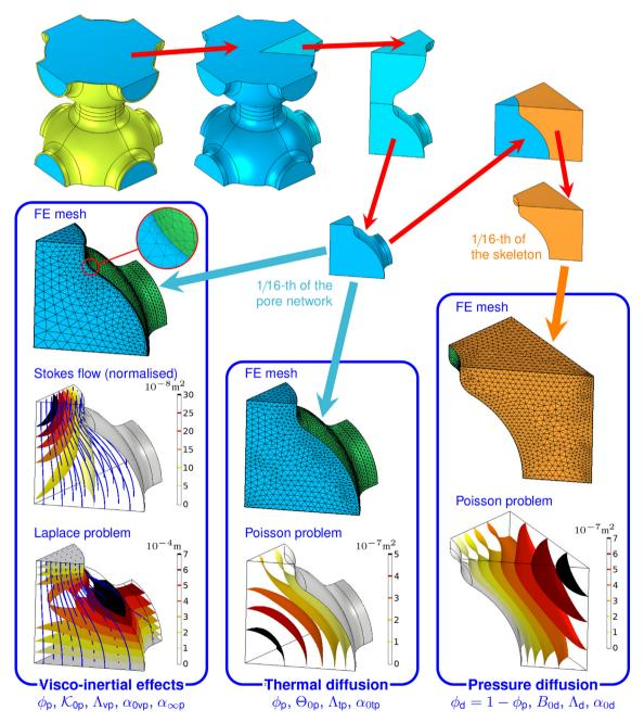
**Fig. 5.** Pore network size correction (yellow parts are removed in the process) and symmetrical slicing, followed by finite-element calculations of macro-parameters related to micro-scale phenomena. (For interpretation of the references to colour in this figure legend, the reader is referred to the web version of this article.)
