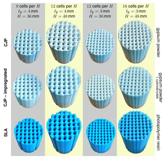
Fig. 3. Additively manufactured samples.
