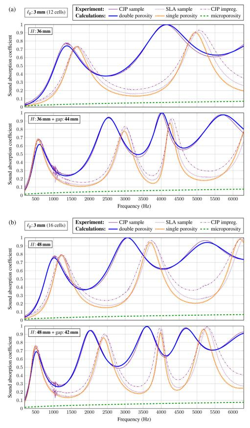
Fig. 9. Predicted and measured sound absorption for single- and double- porosity samples (backed with a rigid wall or an air gap) with a periodic cell size of  $\ell_p = 3$  mm and a height of: (a) H = 36 mm, and (b) H = 48 mm.
