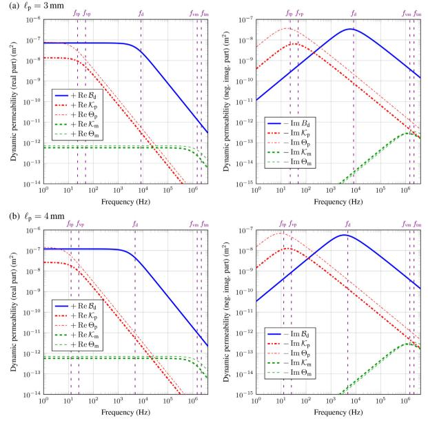
**Fig. 6.** Dynamic permeabilities related to the visco-inertial effects, thermal diffusion and pressure diffusion in the examined double-porosity medium (i.e. assuming the pore networks of CJP samples) with a periodic cell size of: (a)  $\ell_p = 3$  mm, (b)  $\ell_p = 4$  mm.
