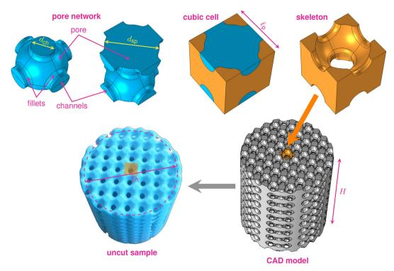
**Fig. 2.** Top row: periodic pore network (two views vertically shifted by half the cell size,  $\frac{1}{2}\ell_p$ ), the corresponding representative cubic cell and skeleton. Bottom row (from right to left): CAD model of a cylindrical specimen and the resulting 3D-printed sample ( $\ell_p = 4\,\mathrm{mm}$  and  $H = 36\,\mathrm{mm}$ ) with a diameter slightly larger than the required size  $D_t = 29\,\mathrm{mm}$  (to be cut so that it fits tightly into the 29-mm impedance tubes).
