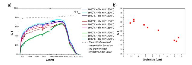
**Figure 3-** (a) Transmission spectra of  $Y_3NbO_7$ : $Ho^{3+}$  transparent ceramics according to sintering conditions (HIP dwell time was 1 h); (b) evolution of the maximum transmission levels at 2  $\mu$ m as a function of grain size.
