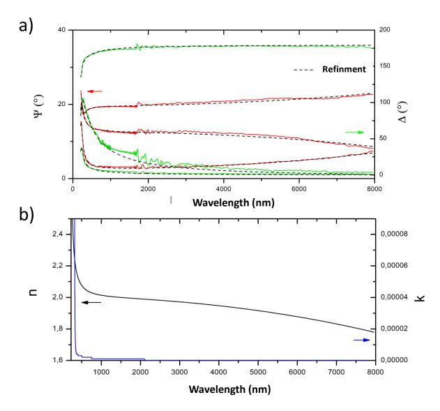
Figure SI2- n refractive index dispersion and k attenuation coefficient of  $Y_3NbO_7$ :  $Ho^{3+}$  ceramics.
