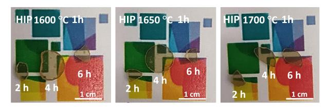
**Figure 1-** Optical micrographs of  $Y_3NbO_7$ : $Ho^{3+}$  transparent ceramics after HIP and reoxidation as a function of sintering conditions. The temperature of the 1 hour HIP treatment is indicated on the top of the picture. 2h, 4h and 6h indicate the dwell times of the natural sintering step at 1600°C, applied after shaping by CIP.
