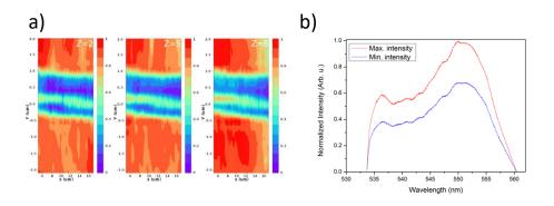
Figure SI3- Microluminescence mapping obtained under a 450 nm excitation and corresponding to the integrated  ${}^5F_4, {}^5S_2 \rightarrow {}^5I_8$  visible transition: a) 3D mapping of  $Y_3NbO_7:Ho^{3+}$  with different z values (3 depths), b) Spectral distribution obtained in the lowest and highest intensity area (blue and red curves respectively) of the  $Y_3NbO_7:Ho^{3+}$  pellet.
