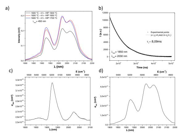
**Figure 5-** (a) Luminescent characterizations of Y<sub>3</sub>NbO<sub>7</sub>:Ho<sup>3+</sup> emission as function of the HIP temperature (same pre-sintering at 1600°C-4 h). (b) Decay curve of the maximal emission. (c) Estimated absorption cross section and (d) calculated emission cross section of the sample. These last characterizations were performed on the sample pre-sintered 4 h at 1600°C.
