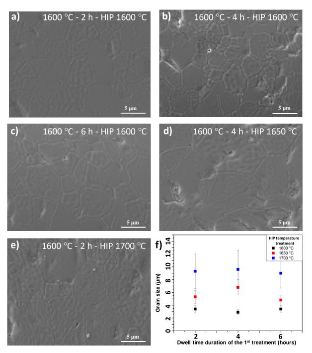
**Figure 2-** (a-e) SEM micrographs of polished and thermally revealed surfaces of  $Y_3NbO_7$ : $Ho^{3+}$  ceramics and (f) evolution of the grain size as a function of the sintering conditions (temperature and time of pressureless sintering and post-HIP temperature with a dwell time of 1 h).
