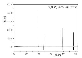
**Figure 4-** X-Ray diffraction pattern of the ( $1600^{\circ}$ C-6hours, HIP  $1700^{\circ}$ C) pellet for which the lowest transmission is observed. This pattern confirms the absence of phase decomposition as all the peaks are attributed to the  $Y_3$ NbO<sub>7</sub> compound (indexation with the 00-036-1353 JCPDS file).
