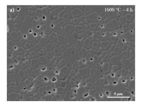
Figure SI1- Ho<sup>3+</sup>-doped Y<sub>3</sub>NbO<sub>7</sub> heat –treated at 1600°C during 4h microstructure
