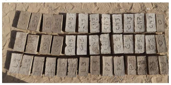
Figure 11: Samples of bricks prepared using a variety of stabilizers and dosages. © T. Joffroy
