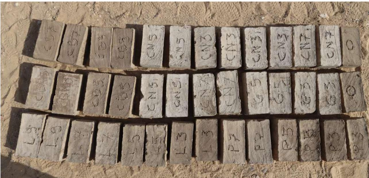
Figure 11: Samples of bricks prepared using a variety of stabilizers and dosages.
