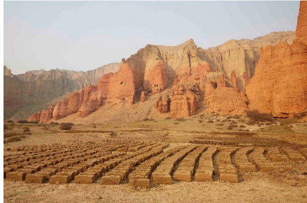
Adobe (sundried mud bricks) production site near Drakmar, Upper Mustang
