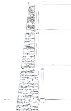
Dry stone masonry walls, with thicker base for stability. Detail from house documentation, Gatlang, Rasuwa, 2018 – ©CRAterre
