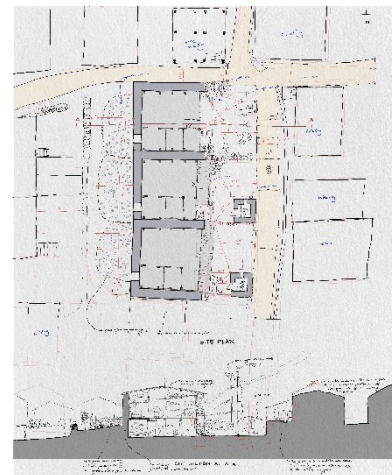
The houses are usually built on horizontal terraces where groups of three to five detached houses are located. The slope does not favor façades facing south, so the main openings in the houses face to the southeast, with ample space between one row and another, permitting solar gains —© ASF Nepal
