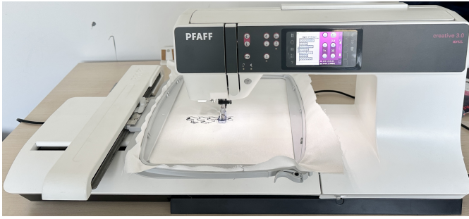
Fig. 2: The embroidery machine is embroidering a chart. Notice the hoop that holds and stretches the fabric for the embroidery process.
