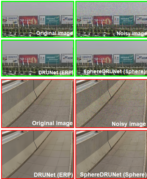
Figure 5: Zoomed portions of the mollweide projection of the Equirectangular image denoised by the DRUNet that was re-trained on ERP images and the Spherical image denoised by our SphereDRUNet. AWGN of \sigma = 30/255 was added on the original image.
