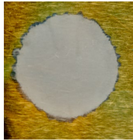
Fig. 1 The photo of a thin target (target #4) made by co-electrodeposition technique. The thickness is 18 \mu\text{m} and the diameter of the deposit is 1.5 cm.
