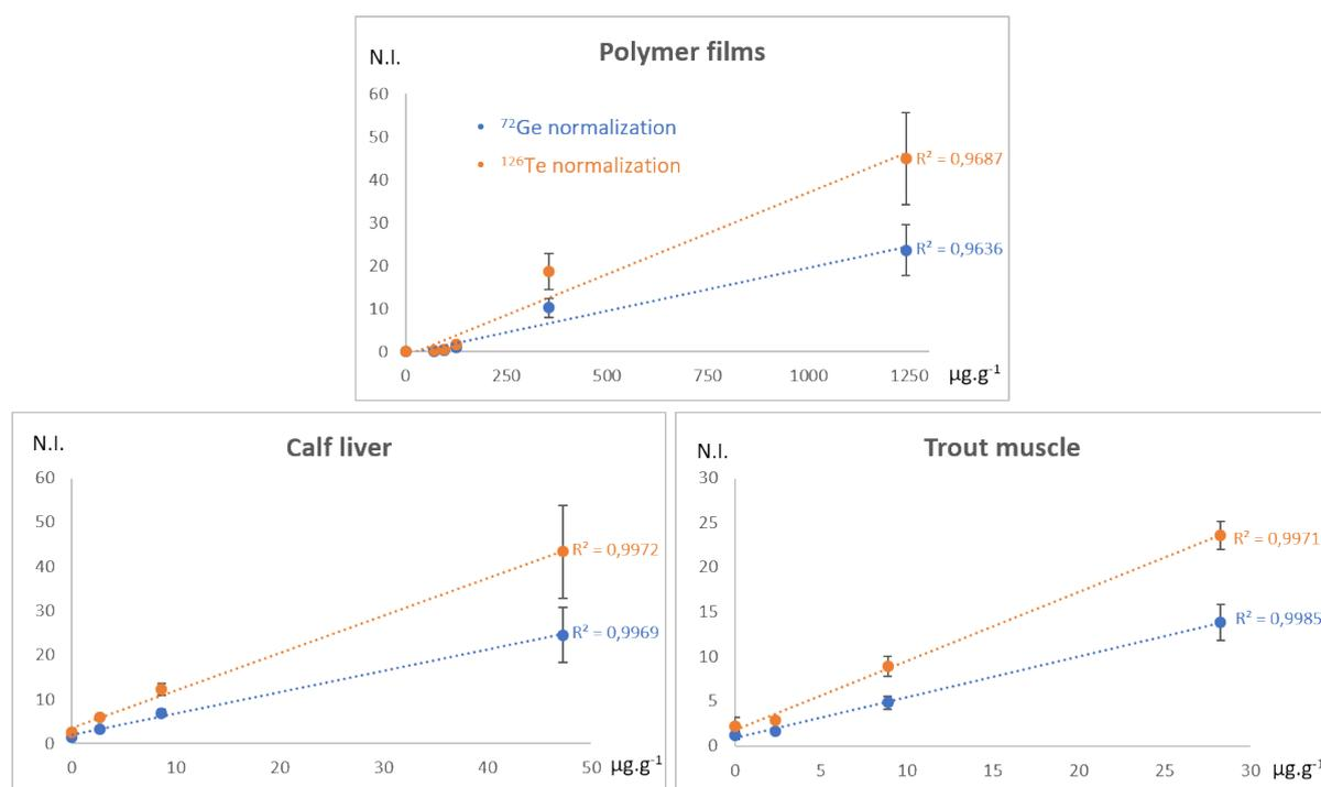
**Fig. 1.** Examples of Hg calibration curves obtained by the LA-ICP MS analysis of polymer films, of trout muscle and of calf liver standards. Intensities are normalized by  $^{72}\text{Ge}$  or by  $^{126}\text{Te}$ , and are plotted as a function of the experimental concentrations.
