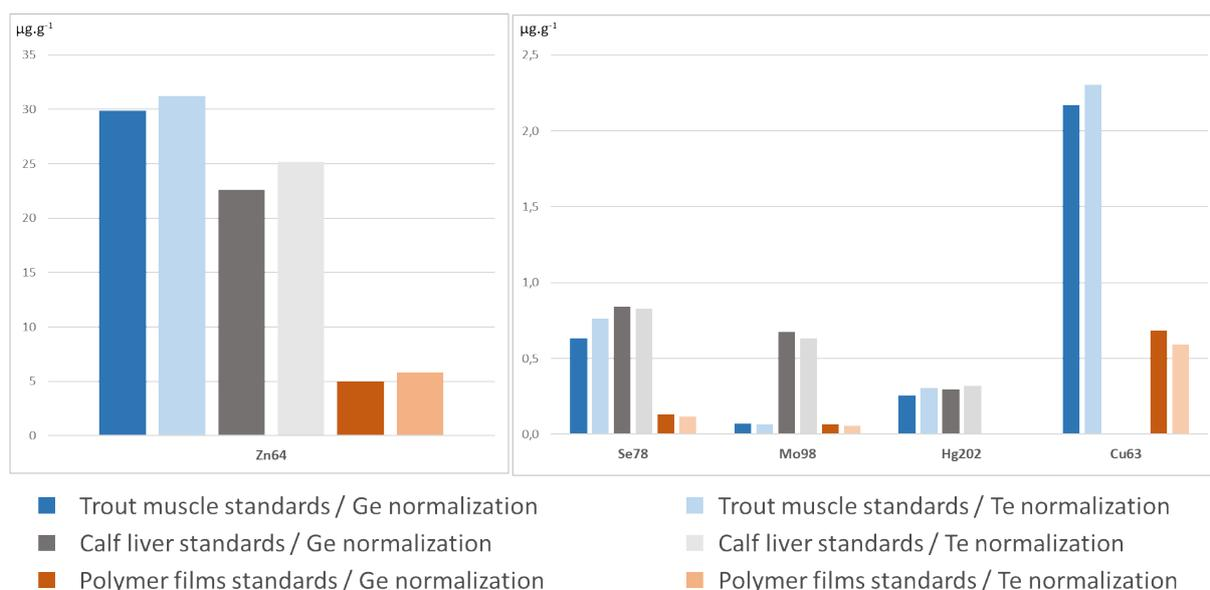
**Fig. 3.** Limits of detection ( $\mu\text{g}\cdot\text{g}^{-1}$ ) obtained with the polymer films standards (orange), with trout muscle standards (blue) and with calf liver standards (grey), and after Ge normalization (darkest colour) and Te normalization (lightest colour).
