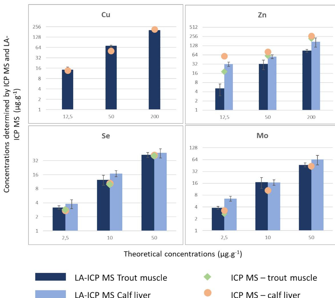
**Figure 4.** Metal concentrations determined by LA-ICP MS with the polymer films method (histogram) and by ICP MS (dots) in trout muscle (LA-ICP MS: dark blue; ICP MS: green) and calf liver (LA-ICP MS: light blue; ICP MS: orange) standards (log scale),  $n = 11$  analysis.
