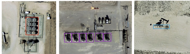
Fig. 2: Example of images and annotated objects from OG database : tank (red), compressor (purple) and well (blue) source : @Google Earth
