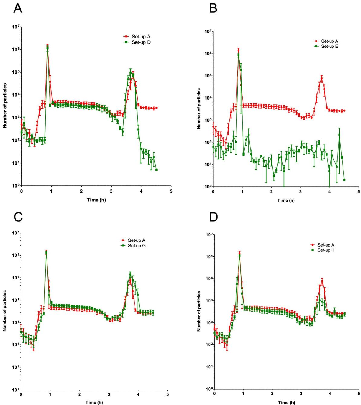
**Figure 5.** The particle distribution over time, showing the impact of in-line filtration and the hydration position on the particulate load in set-up D (A), set-up E (B), set-up G (C), and set-up H (D). The results are expressed as the mean  $\pm$  SD ( $n = 5$  or 6).
