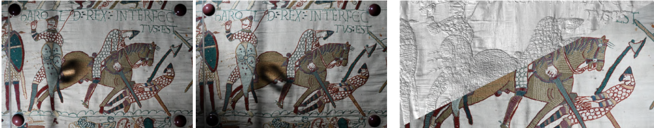
(a) Two of the input images. Note the shadows and caustics induced by the spheres and the glass. (b) Highly detailed 3D-reconstruction, overlaid on one pre-processed input image.
