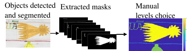
Figure 13: Setting each element’s average height, from the detected and segmented masks. Here the background is at level zero, the letters at 2 mm, and the comet at 3 mm.
