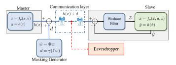
Fig. 2. Scheme of the proposed masking/de-masking protocol.
