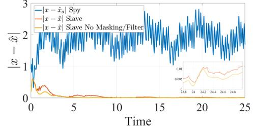
Fig. 4. Evolution of the adversarial observer (Spy) error norm,  $|x - \hat{x}_a|$ , and the error norm of the slave with the washout filter,  $|x - \hat{x}|$  and the error norm of the same slave without the masking/filter architecture.
