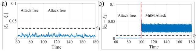
Fig. 5. a) Evolution of the norm  $|\xi_1 - \hat{\xi}_1|$  of the first 6 states of  $\xi$ . b) Evolution of the norm  $|\xi_1 - \hat{\xi}_1|$  of the last 6 states of  $\xi$ . At 100 seconds there is a man-in-the-middle (MitM) attack in the transmitted signal,  $y_2$ .
