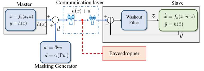
Fig. 2. Scheme of the proposed masking/de-masking protocol.
