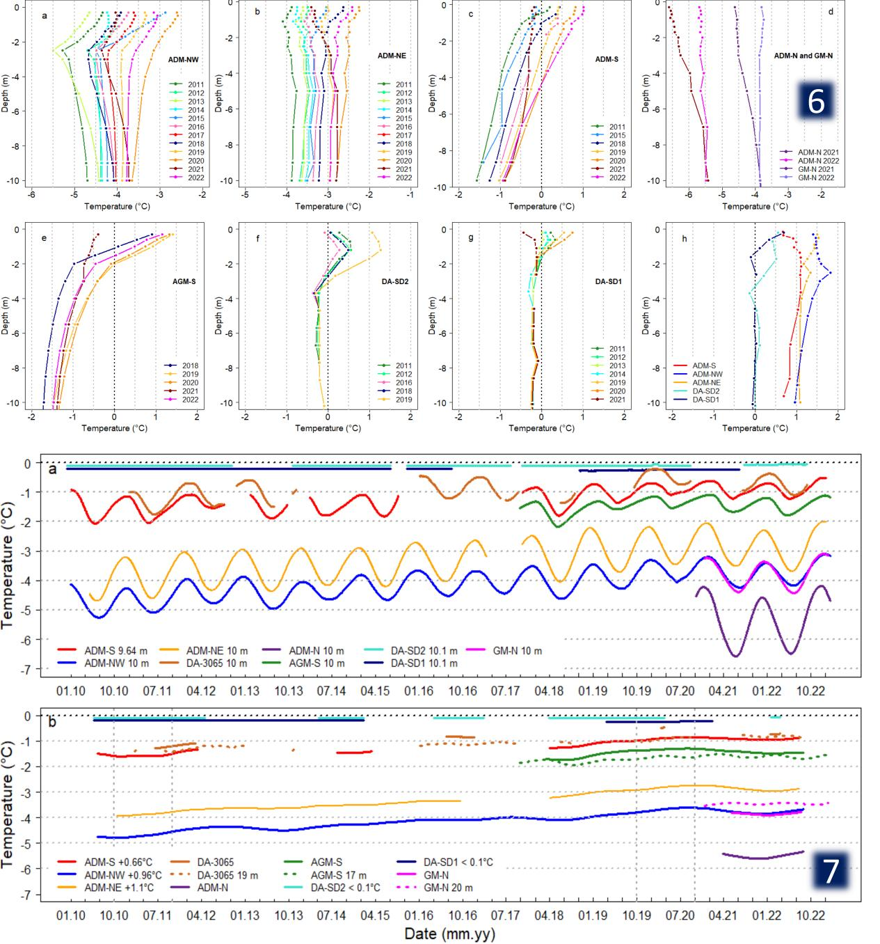
Mean annual Temperature-depth (Tz) profiles are calculated for available hydrological years at and each borehole (Fig. 6 a-g) and decadal trends (2011-2020) are calculated with linear regression from annual means (Fig. 6h). Daily temperature at 10 m depth and deepest sensor when available is displayed with a 31-day running mean (Fig. 7a) and a 365 running mean (Fig. 7b). Decadal trends are calculated from linear regressions.
