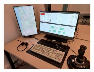
Fig. 2. Experimental setting composed of two screens, one custom keyboard, one joystick and a headset
