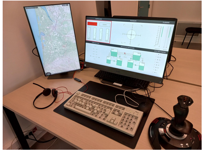
Fig. 2. Experimental setting composed of two screens, one custom keyboard, one joystick and a headset
