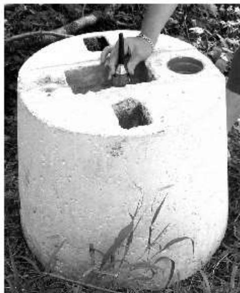
Fig. 2. Concrete block of 300 kg and its hydrophone.
