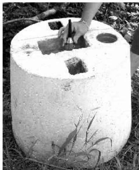
Fig. 2. Concrete block of 300 kg and its hydrophone.
