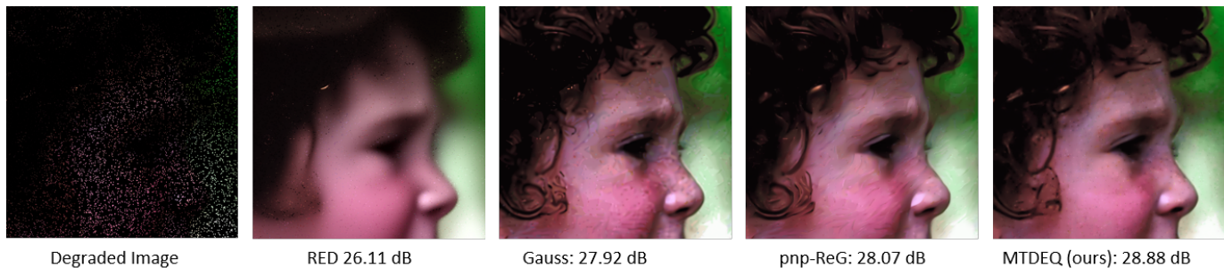
(b) Example of Gaussian deblurring with \sigma_{\text{blur}} = 1.6 and \sigma_{\text{noise}} = 0.01 .
