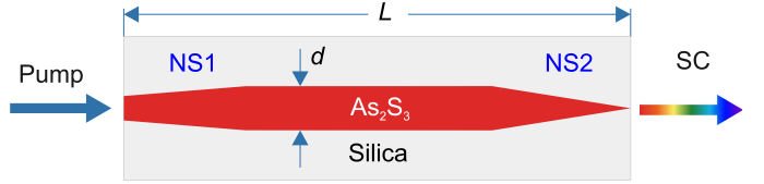
Fig. 2. The structure of the \text{As}_2\text{S}_3 -silica hybrid waveguide. Two nanospikes are integrated at both waveguide ends.
