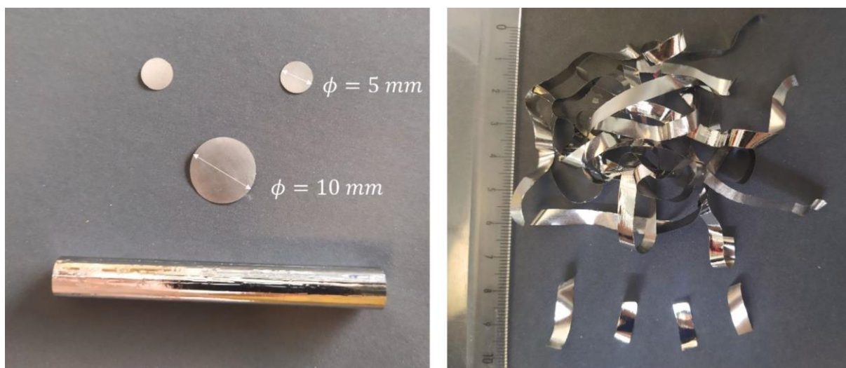
Fig. 1. Metallic glasses synthesized into rod shape (left) and ribbon shape (right).
