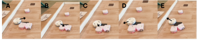
Fig. 12. Emerging attack behavior in C4 : (A) the robot is confronted to two predators blocking a resource. (B) the robots turn in the direction of the predators. (C) The robot repulses one of the predators, accessing the resource. (D) The robot turns to escape.
