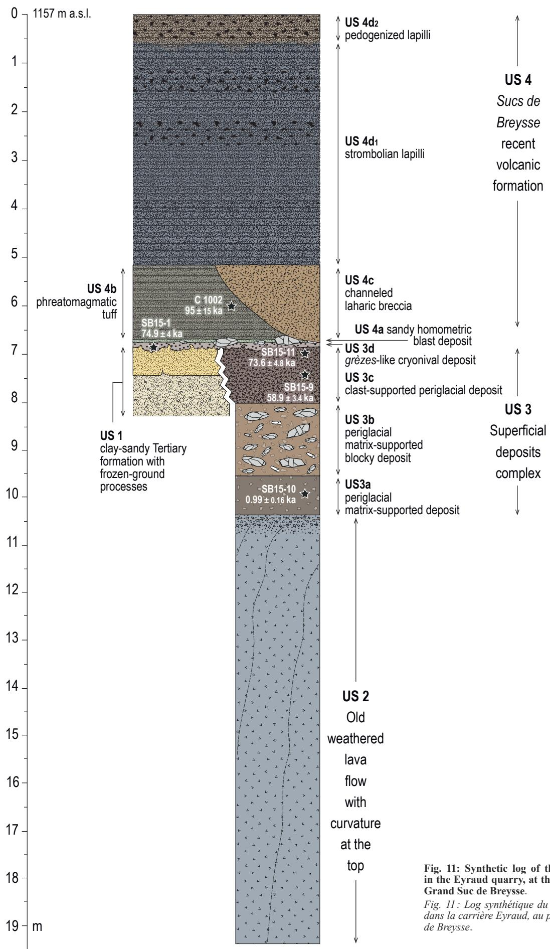
Fig. 11: Synthetic log of the observable setup in the Eyraud quarry, at the eastern foot of the Grand Suc de Breysse.
