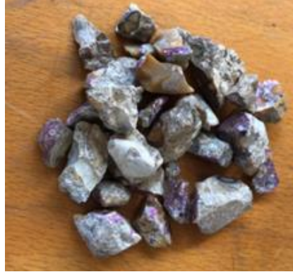
Fig. 3 recycled concrete aggregates
