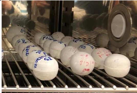
Fig. 1 4 cm diameter mortar spheres (modeling material).
