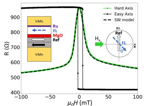
**FIG. 1.** Resistance vs magnetic field of a  $4 \mu\text{m}$  diameter circular junction with 0.3 nm Ru spacer. Magnetic field is applied along easy (black) and hard (green) axes. The dashed line is the fit using the Stoner Wohlfarth model with  $\mu_0 H_{ex} = 2.6 \text{ mT}$ ,  $\mu_0 H_k = 6.6 \text{ mT}$ ,  $\mu_0 H_R = 450 \text{ mT}$ , and  $\delta = 4.05^\circ$ . Insets: side view (left) and top view (right) of the magnetic tunnel junction.
