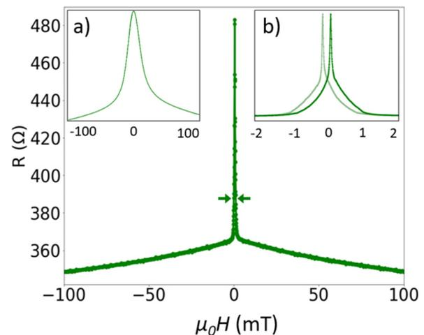
**FIG. 5.** Response curve of a circular junction with  $\mu_0 H_{ox} = 4.75$  mT, before (a) and after the deposition of the flux concentrator. The response curve's slope is much steeper (corresponding to a sensitivity of 543%/mT) due to the high field amplification. A zoom of this curve is shown in (b) for increasing (dark) and decreasing (light) magnetic field sweep.
