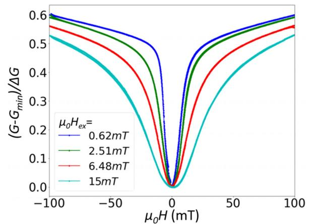
**FIG. 2.** Normalized conductance measured under 100 mV voltage bias, as a function of magnetic field applied along the hard axis ( $x$ -axis) for several 4  $\mu\text{m}$  diameter circular junctions with decreasing values of free layer exchange field. The 15 mT exchange field corresponds to a direct contact of the free layer with the antiferromagnet (no Ru spacer).
