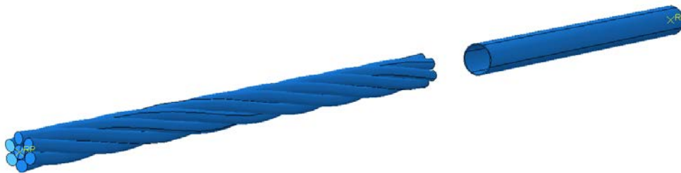
Fig. 13. Initial position of the model with combined stress using optimal meshing parameters
